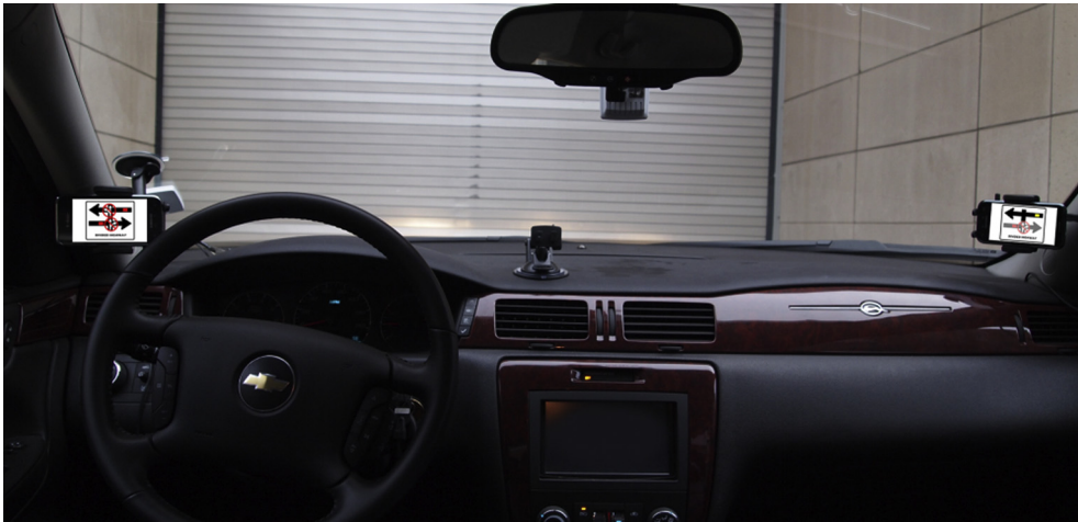
Fig. 2. The location of the displays for the in-vehicle intersection crossing system.
