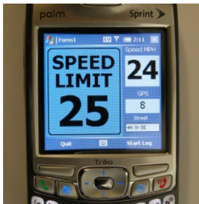
Figure 4-5. A blue speed limit sign indicates a reduced speed limit is in effect due to weather conditions.
