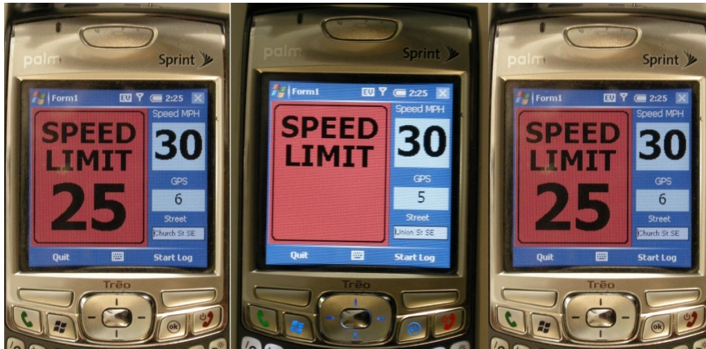
Figure 4-4. A red flashing speed limit sign indicates the driver is speeding. Actual speed is shown in the top right corner of the display.
