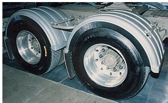
Figure 3. A depiction of the Dynaplas Pty. Limited full wheel mudguards and spray suppressant kit.
