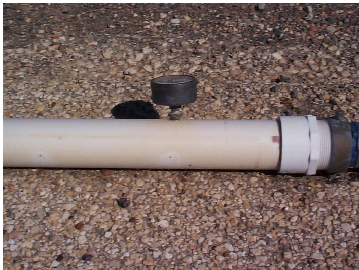
Figure 8. Depiction of the 2 inch (5.08 cm) PVC pipe perforated with holes at six inch (15.24 cm) intervals.
