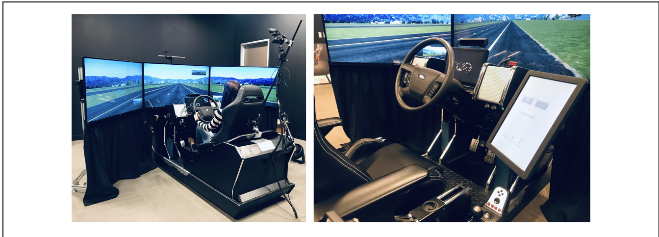
Figure 1. The driving simulation lab setup. The left figure shows the driver's seat and forward view screens, and the right shows the dashboard and the automated system console (the tablet screen to the right of the steering wheel). Note that the eye-tracking system is positioned on top of the dashboard.
